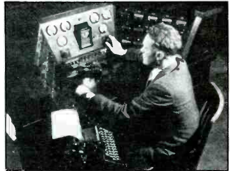
Chief Transmitter Engineer J.E. Whitehouse operates the master transmitter control console at WLW/W8XO. It also controlled other local Crosley stations WSAI and shortwave W8XAL.
