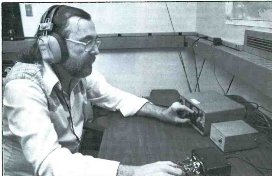
ARRL Lab Engineer Ed Hare, KA1CV, tunes the bands with his Heathkit HW-7. This venerable QRP rig has been modified to put out only 9 milliwatts! So far, Ed's been able to work 25 states and a handful of DXCC countries with his extremely low-power rig.
