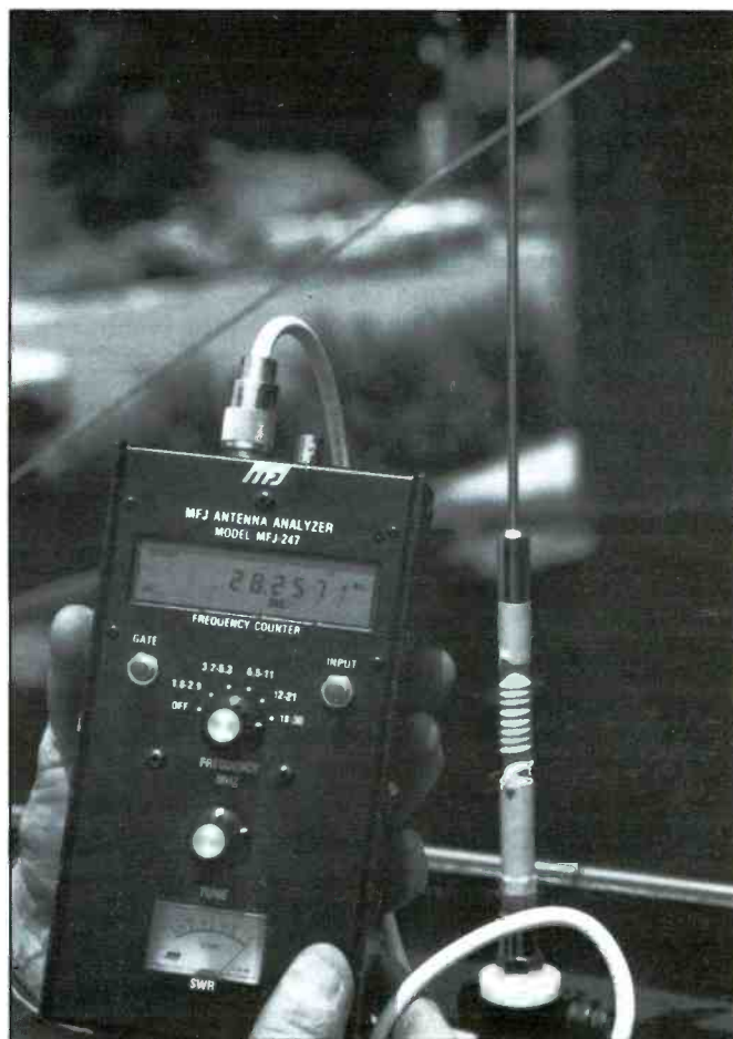
The MFJ SWR analyzer is a fast and easy way to fine tune a whip.
